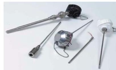
The millivolt potential that is created in the thermocouple conductors differs depending on the materials used. Some materials make better thermocouples than others because the millivolt potentials created by these materials are more repeatable and well established. These thermocouples have been given specific type designations such as Type E, J, K, N, T, B, R and S. The type of T/C used also depends on temperature monitored and environment.
